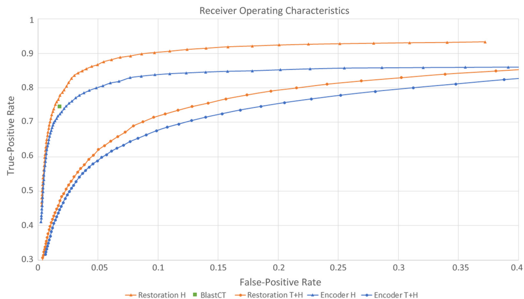
Fig. 7 ROC curves for two test datasets (H, hemorrhage; T+H, tumor and hemorrhage) for two network versions (restoration and encoder). The result for the hemorrhage detection tool BlastCT 20 is marked as a point.
