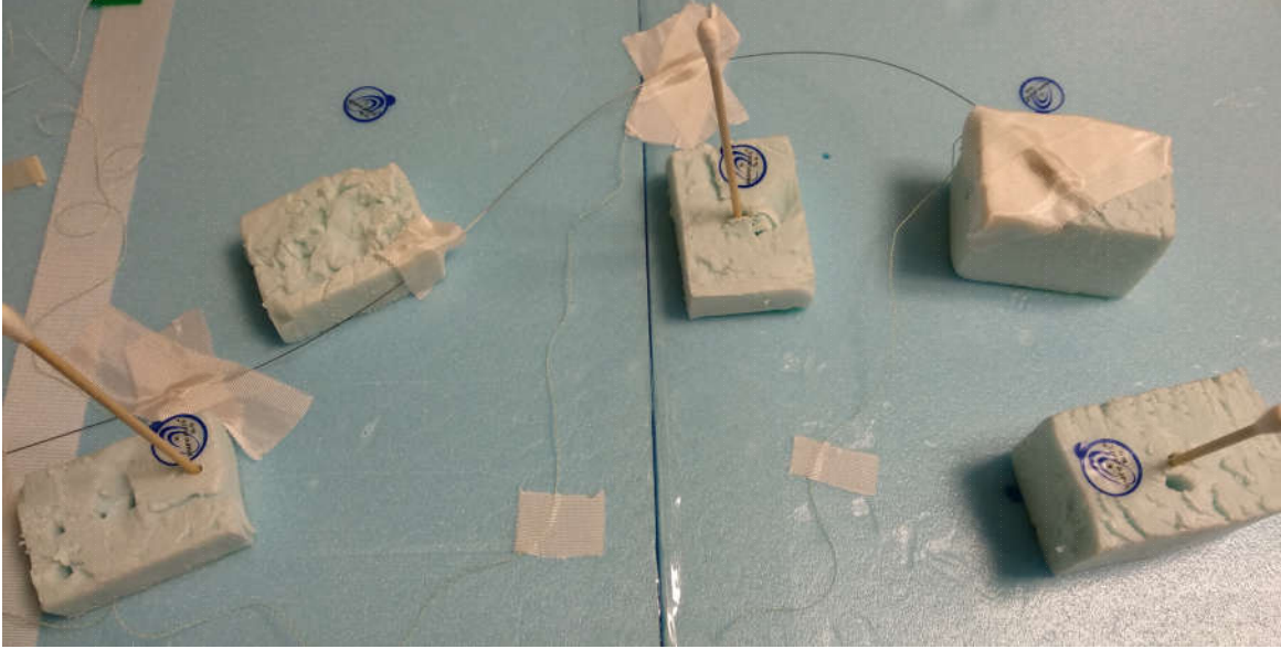
Figure 4. A picture of the 3D curve experiment showing the fixed catheter prototype and the metallic markers. The EM sensors were fixed with double sided tape and surgical tape to ensure no movement of the EM sensors and the optical fiber.
